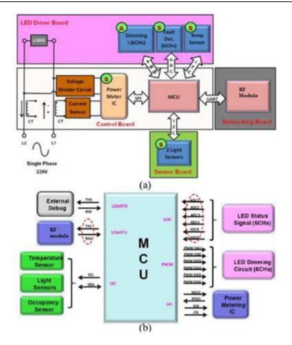
Fig. 2. Proposed LED smart lamp. (a) Monitoring system block diagram. (b) Block diagram of microcontroller unit interface
